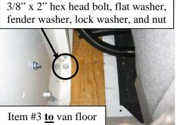
Secure the **Front Bulkhead**. Drill (2-one per-side) 3/8" holes through the frame, ½" plywood, and floor of vehicle Attach using 3/8" x 2" hex head bolt, flat washer, fender washer, and nut.
